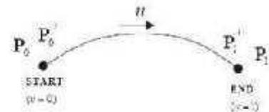
$$P(u) = [1 - 3u^2 + 2u^3 \quad 3u^2 - 2u^3 \quad u - 2u^2 + u^3 \quad -u^3 + u^4] \begin{bmatrix} P_0 \\ P_1 \\ P'_0 \\ P'_1 \end{bmatrix} \quad \text{: Hermit curve}$$
